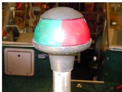
This combination bow light fixture with a cloudy lens is a candidate for replacement with an LED combination fixture, or better yet, a pair of individual red and green fixtures.
