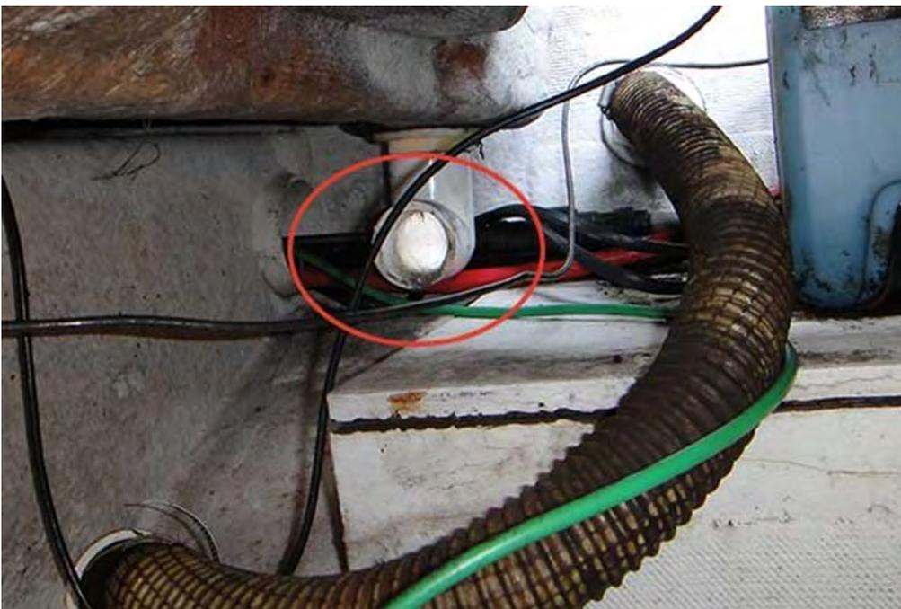
This cockpit drain leads not overboard, but right to the bilge, relying on the bilge pump to keep the boat afloat—this boat should only be left unattended while pulled out or on a lift.
