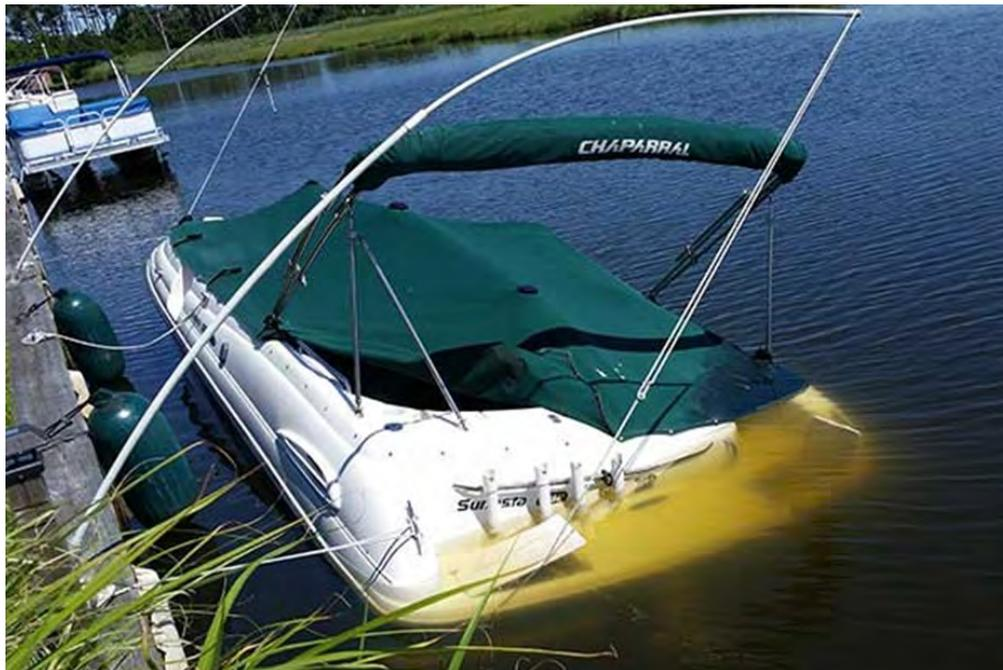
The cover on this boat filled with rainwater, and because the scuppers were already at the waterline, they back-flooded, and the boat sank.
